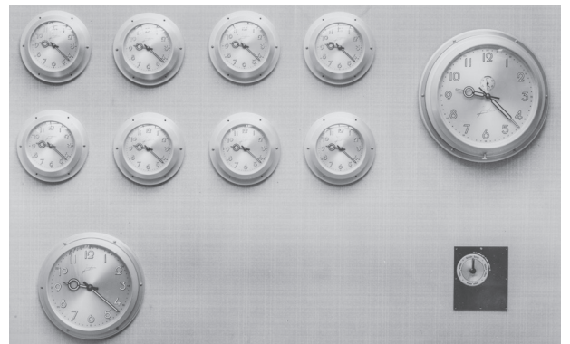
Junghans Airship Clock System from 1935, consisting of a main clock and several auxiliary clocks.
