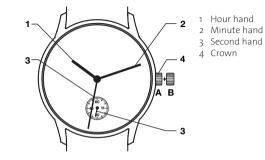
With the crown in position A, you can wind up the hand-winding movement by turning the crown. Maximum accuracy and power reserve are guaranteed when the movement is fully wound.
